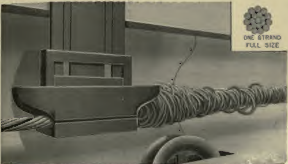
RESULT OF A BROKEN STRAND.
